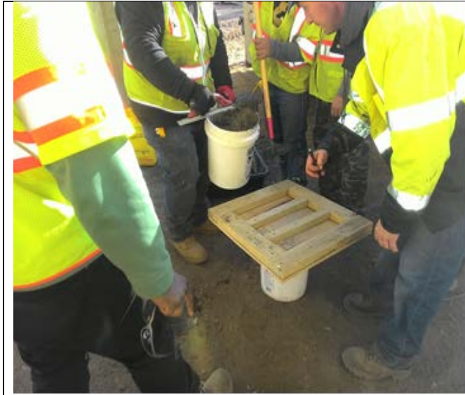
Placing Pigment and SIKA 123 mixture into form for Coloration Sample
