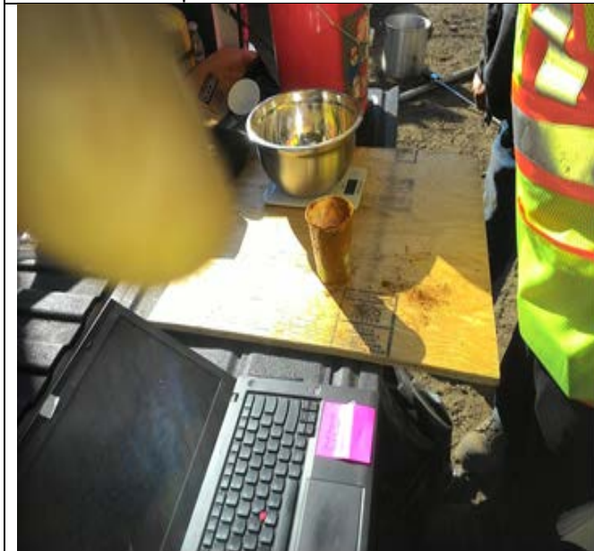
Handon weighing pigment material to mix with SIKA 123 for sample batch
